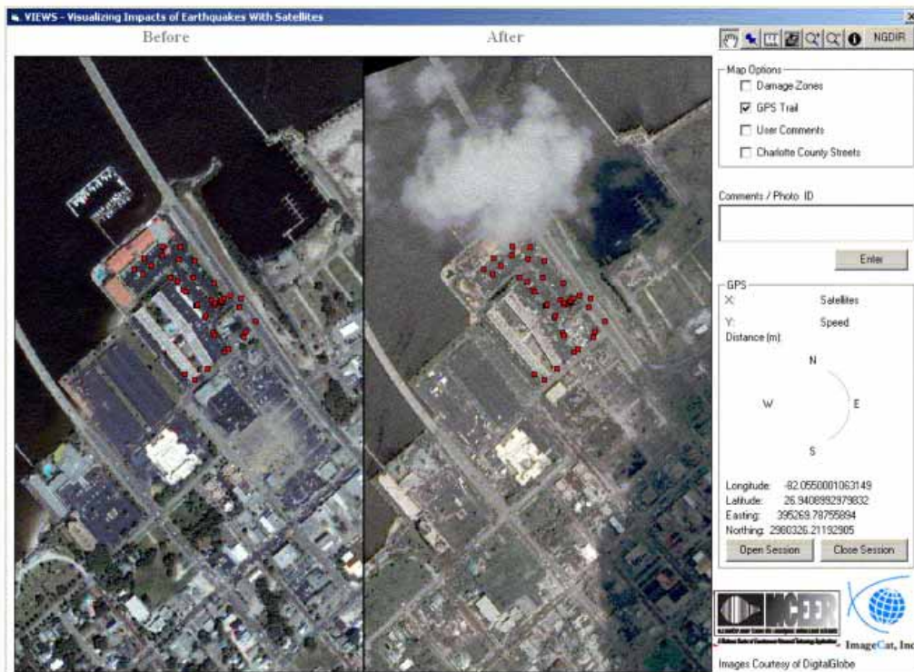
Figure 3. User interface for the VIEWS system, deployed to collect building damage data in Punta Gorda and Port Charlotte after Hurricane Charley. Quickbird satellite images acquired 'before' and 'after' the hurricane form the base layer, which is overlaid here with GPS readings for one of the routes taken.
