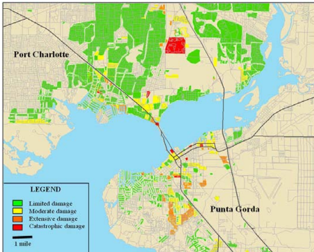
Figure 5. Post-hurricane damage zones in Charlotte County published by FEMA on August 20, 2004.
