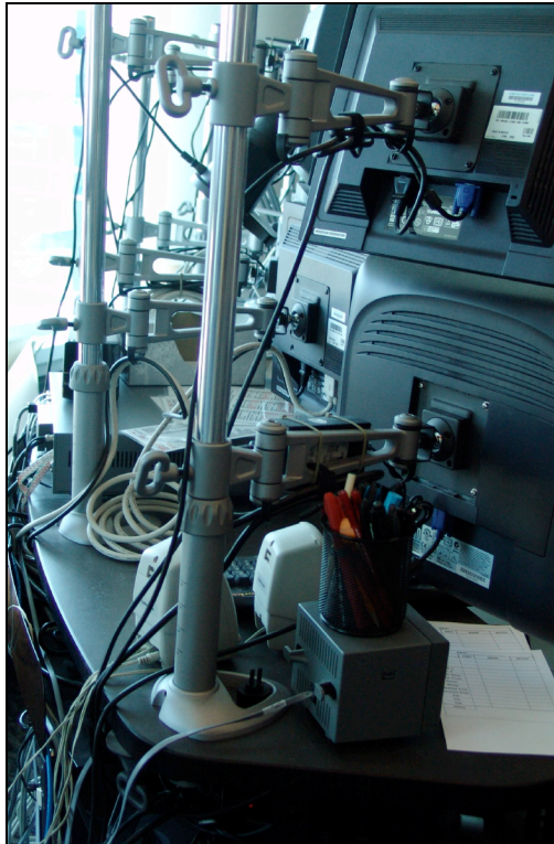
Fig. 13. Restraints on computer screens
