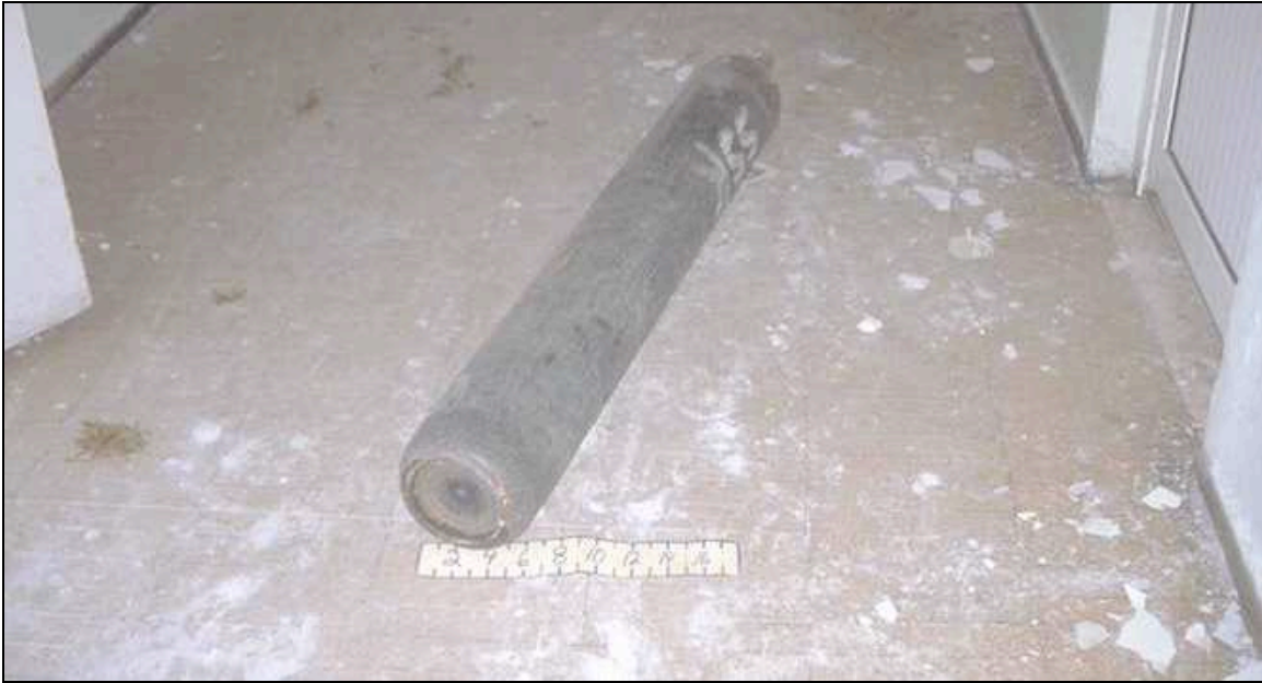
Fig. 8. Unrestrained cylinder toppled over.
