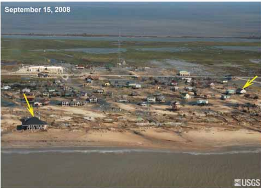
USGS photo of Bolivar Peninsula, Texas, Sept. 9 (top) and Sept. 15, 2008, two days after landfall of Hurricane Ike (bottom). Yellow arrows mark features that appear in each image. Photo shows loss of houses, eroded dune face, and sand deposited inland. http://coastal.er.usgs.gov/hurricanes/ike/photo-comparisons/bolivar.htm
