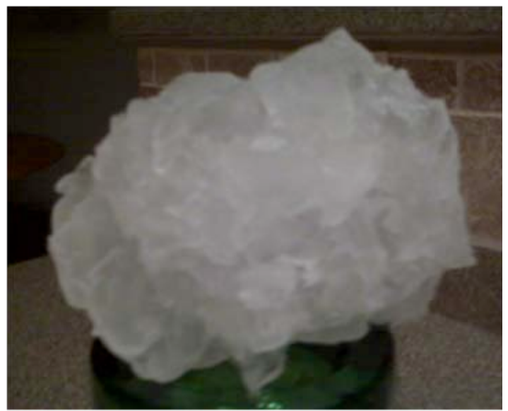
Figure 3a: A real hailstone collected by Texas Tech severe storm researchers during VORTEX 2 2009. Figure 3b: An artificial hailstone created by IBHS researchers.
