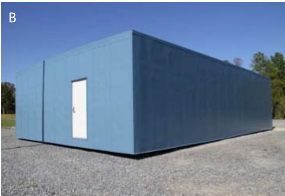
Figure 2: The a) original WERFL building in Lubbock, Texas and the b) replica building for use in testing at the IBHS Research Center in Richburg, SC.
