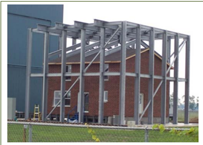
Figure 2: Photograph of the ‘Three Little Pigs’ first test house, surrounded by the steel reaction frame used to hold the wind loading system (not shown).
