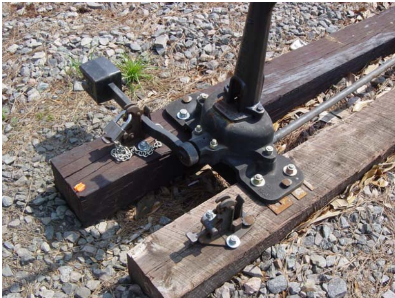
Figure 6. Rail switch: It was the responsibility of the crew who used the side track to set the switch back to the main line.
