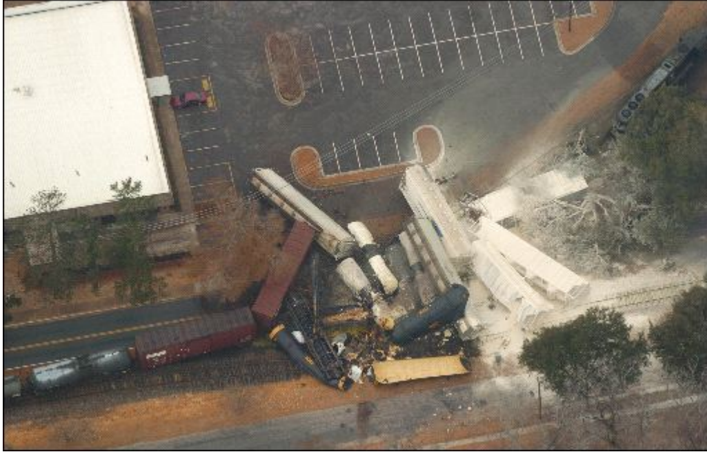
Figure 7. Train derailment: The Columbia, South Carolina, bound train failed to continue on the main track (bottom), veered left onto the side track, and collided with a parked locomotive. Source: Andrew Davis Tucker, Augusta Chronicle
