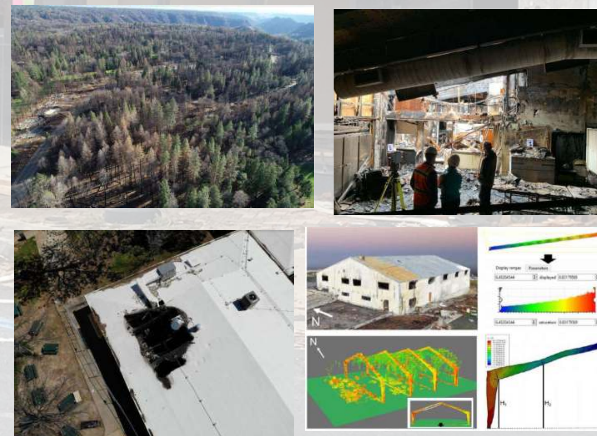
Fig. 6: Camp Wildfire Data Collection and Subsequent Analysis of Damaged Buildings (Schulze et al. 2020)
