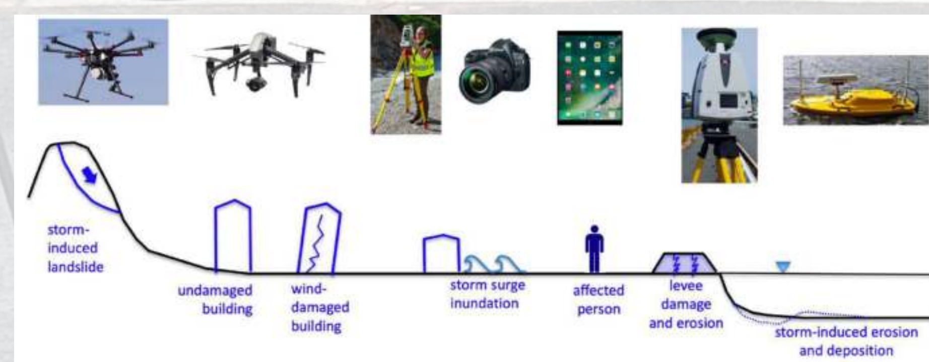
Fig. 3: RAPID Facility Multidisciplinary and Multi-Scale Data Collection (Berman et al. 2020)
